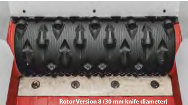
Rotor Version 8 (30 mm knife diameter)
